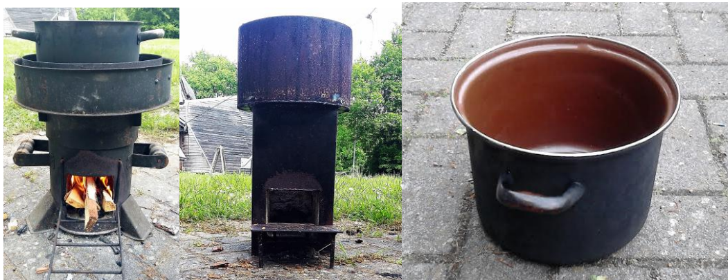
Figure 2. Rocket stove No. 1, Rocket stove No. 2 and pot used during the experiment
