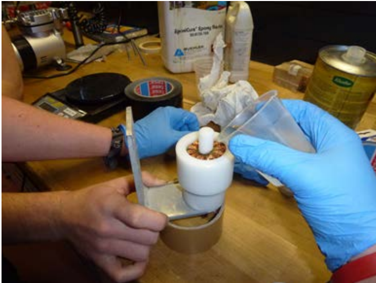
Figure 6: Epoxy resin filling process
