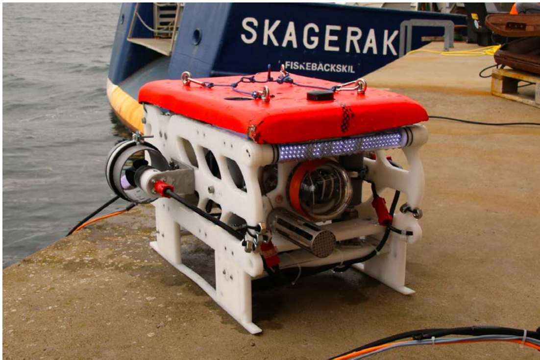
Figure 1: The ROV (length, width, height; 60 cm, 50 cm, 40 cm) of the University of Applied Sciences at the Sven Lovén Centre in Fiskebäcksil, Sweden
